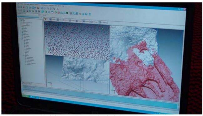
Fig. 2 – Laser scanning of the Hung-e Kamalvand rock relief.
